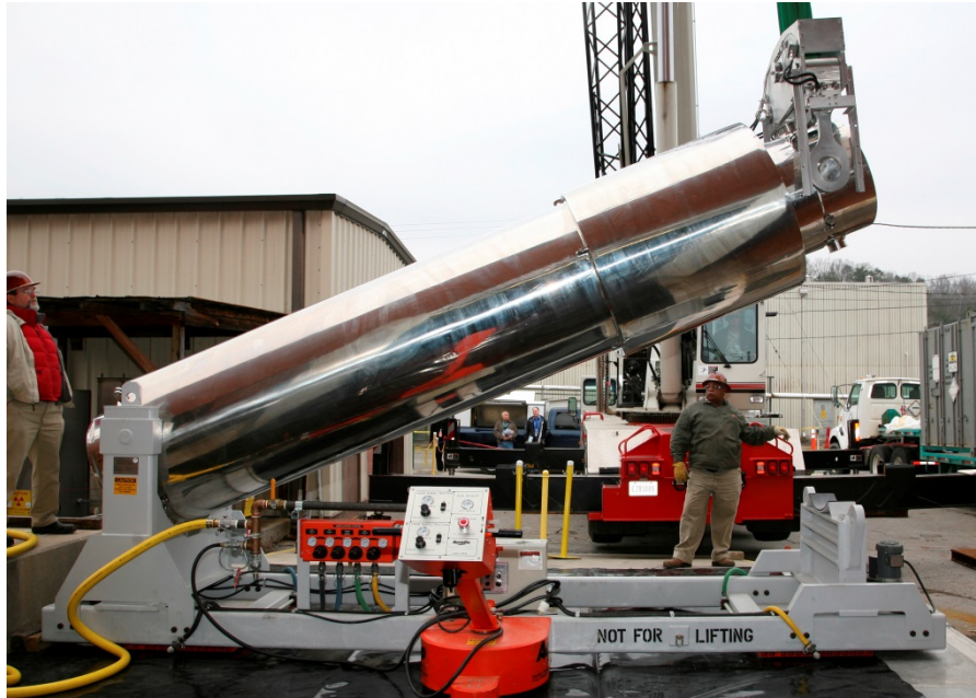
Fig. 6. LWT cask from NAC International set on cradle at ORNL.
